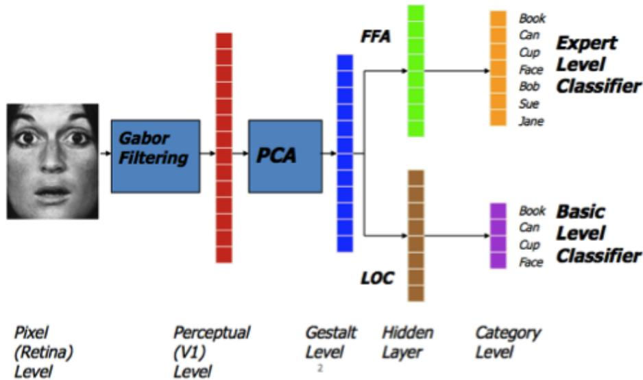
Figure 1: The Model. The first layer is convolutional, using Gabor filters, followed by PCA, followed by a trained hidden layer. The two branches reflect the putative tasks of the LOC and FFA.
